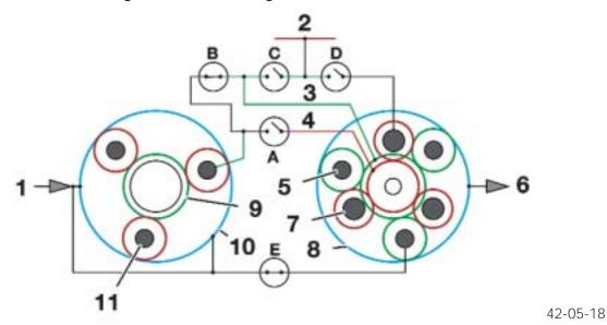
**Power Flow in 6th Gear:** In 6th gear, the sun gear 2 in the double planetary gear train is blocked by clutch C. The planet carrier is driven by the engaged clutch E. As a result, the long planet gears are forced to move by rolling contact (reaction) on the fixed sun gear 2 (3) and drive the internal gear in the direction of engine rotation. *This results in a large gear ratio in overdrive*. The single gear train is not operative in 6th gear.
